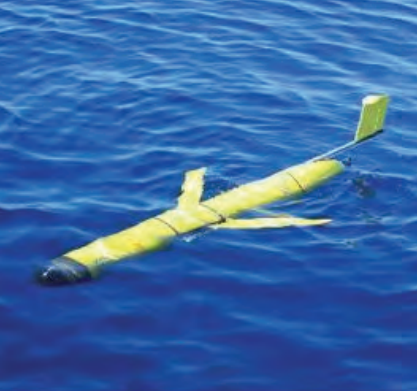
Underwater gliders are used to monitor ocean temperature, salinity, turbidity, chlorophyll, etc.
